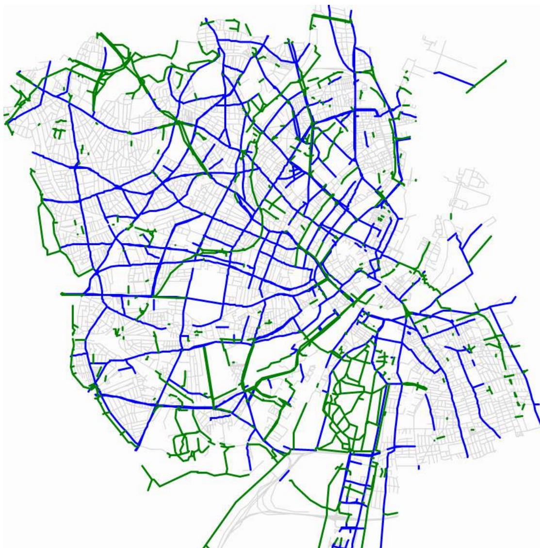
Figure 2.3: The largest connected component of the street network of Copenhagen. Car links are shown in grey, bicycle links in green, multi links (car and bicycle) in blue. The bicycle and multi links (green and blue) together form the bikeable network of protected bicycle infrastructure.
