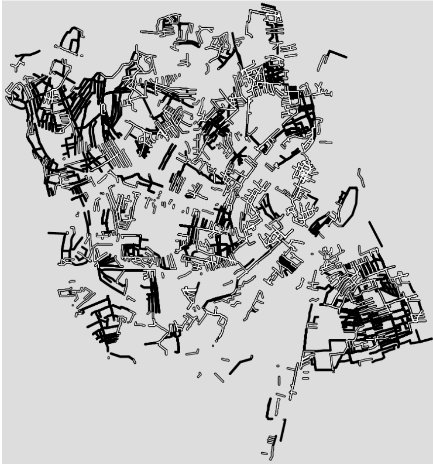
Figure 4.1: Gaps for c_{\text{gap}} = 1200 m are plotted in black. Gaps for c_{\text{gap}} = 500 m are plotted on top, in white and with a thinner line style. All white gaps (smaller cutoff) are contained in the set of black gaps (larger cutoff). Other map details are omitted and the background color is set to grey for the sake of readability.
