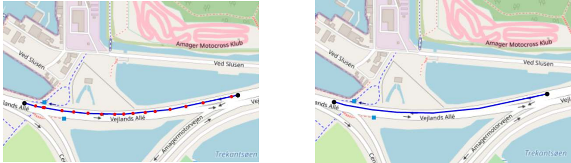
Figure 2.5: Auxiliary nodes in OSM data: Vejlands Allé as example of a curved street. Left: Before simplification, the path between the two black nodes consists of a sequence of 16 auxiliary nodes of degree 2 (red), connected by 17 straight links (blue). Right: After simplification, the path consists of one link, whose curvature in physical space is preserved in the link attribute. [107]
