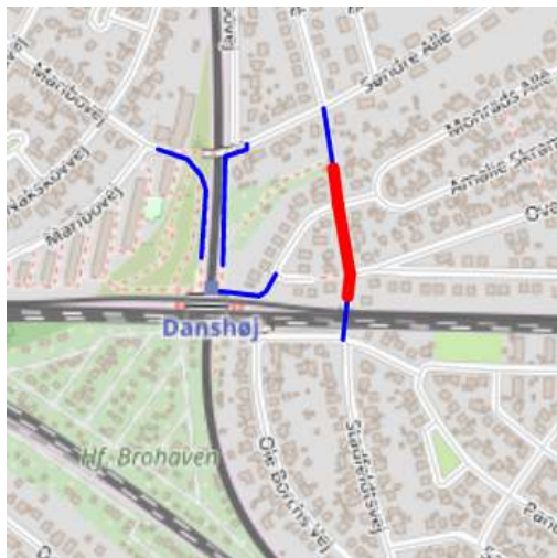
Figure 3.14: Missing links connecting isolated bicycle infrastructure elements: gap 8 on Tschernings Allé (left) and gap 95 on Valløvej (right). [107]
